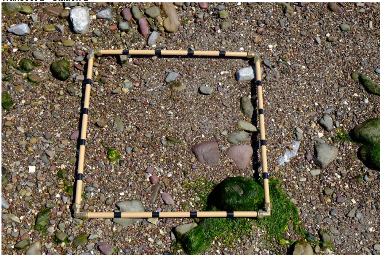
Figure 5. View of beach sediments at Station 2 in quadrat. Quadrat is 50cm by 50cm. Black marks on quadrat frame are at 10cm intervals.
