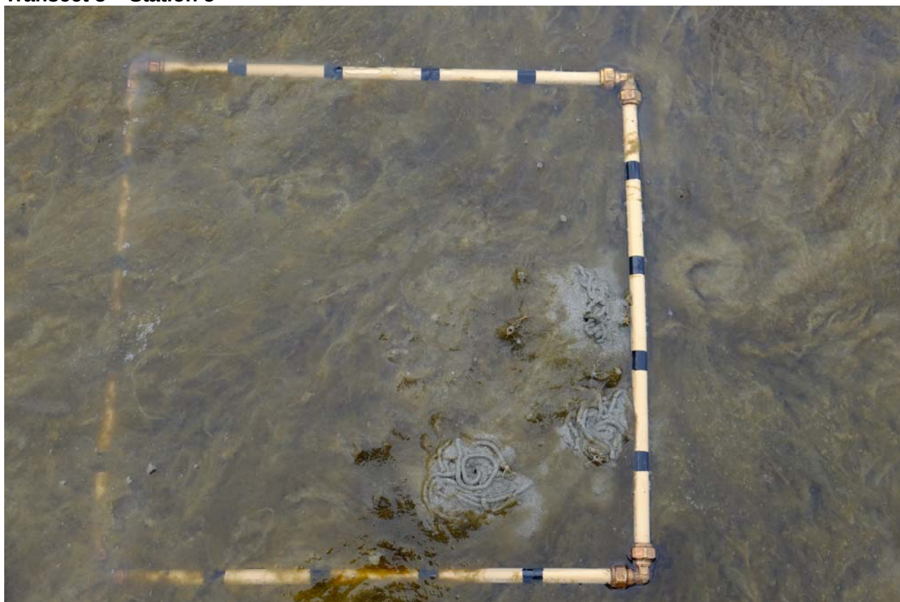
Figure 21. View of beach sediments at Station 5, Transect 3 in quadrat. Quadrat is 50cm by 50cm. Black marks on quadrat frame are at 10cm intervals.
